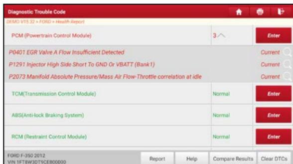
The tested system with fault code appears in red and the system functioning properly displays in black (normally).
